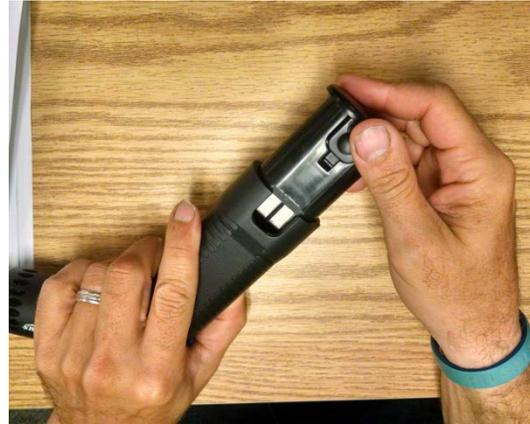
**Figure 4-15. UltraLite ALS Battery Change**
