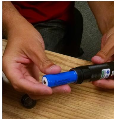
**Figure 3-1. Battery Replacement**
