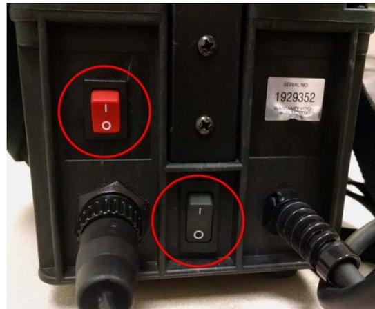
**Figure 4-18. Power Buttons on Battery Pack of Spectroline Maxima**
